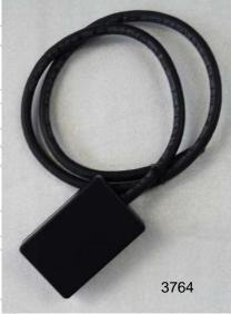
The Bluetooth link will transmit data to a SmartPhone, Tablet, or other handheld device to comply with the requirement for 395.0 for HOS/CSA reporting. These modules have J1939, and Bluetooth interfaces with built-in UTC time stamp and 4 Gbit data storage. They can also collect and store tractor data in non-volatile memory for later download to the Host when connected.
